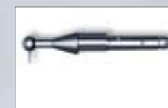
INTRA LUX micro head 22 LB For micro-surgical interventions, such as apicectomies. Maximum operating speed: 20,000 min -1 . 1:1 direct drive ratio. For use with size 2 inverted cone burs. REF 0.549.3650
